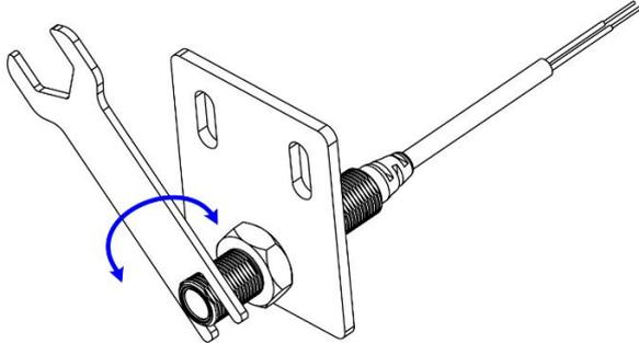
4. Lastly, check if the projected laser line is at the right position to your need. Rotate the laser module again if the laser line isn't aligned with your preferred position.
