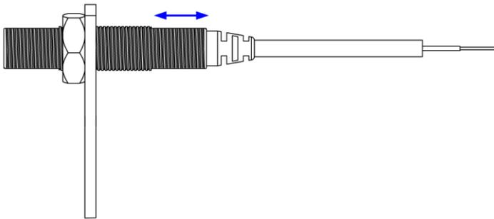
2. Next, tighten the nut with the washer on the plate.
